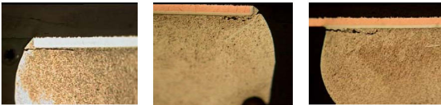
Partial cracks near ball to package interface (not open)
