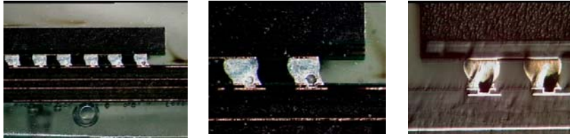
Large voids in solder balls and slight mis-alignment
