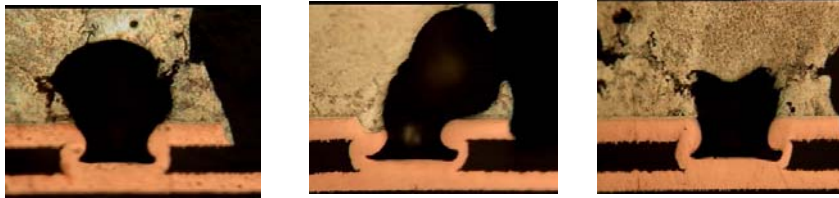
Large voids causing rupture in solder balls
